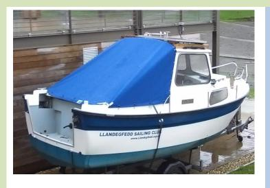
**Penelope** has a new cover which can be unclipped from the transom, rolled up and tied to the cabin roof during racing. We are also fitting a new flag frame and hope to incorporate some form of anti bird netting over the cockpit and cabin. May get an owl too.
