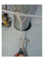
**3** Tie the air block to the mast below the boom vang tang with the piece of 3 mm Vectran (part 10).
