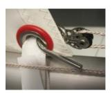
**26** The clew hook can be used as an alternative method of securing the clew of the sail. This may require pliers to open the eye slightly to fit the **micro block** (Part 9).
