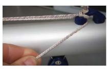
Bring the outhaul line (Vectran V12) back to the boom end feeding it through from the port side.
