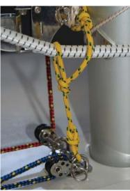
7 Finally tie the mast retention line (part 5) to the tang and the block plate so that the mast can rotate 180 degrees and the bowline acts as a fairlead for the daggerboard bungee below the vang.
