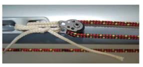
17 Continue to feed the Vectran control line to the block on the boom.
