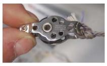
Tie the air block and becket to the end of the Vectran 12.
